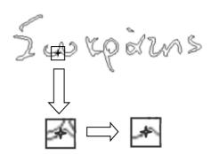
Fig. 4. Local contours in sliding-window. The contours disconnected with the central pixel are neglected, and only the edge fragments connected with center are retained.
